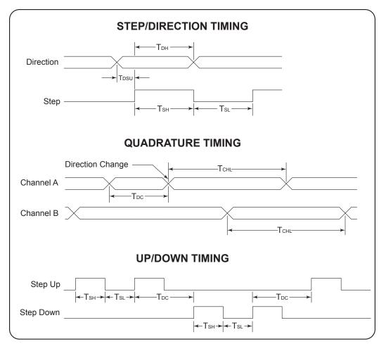
Figure 2.4.3: Clock Input Timing Characteristics
